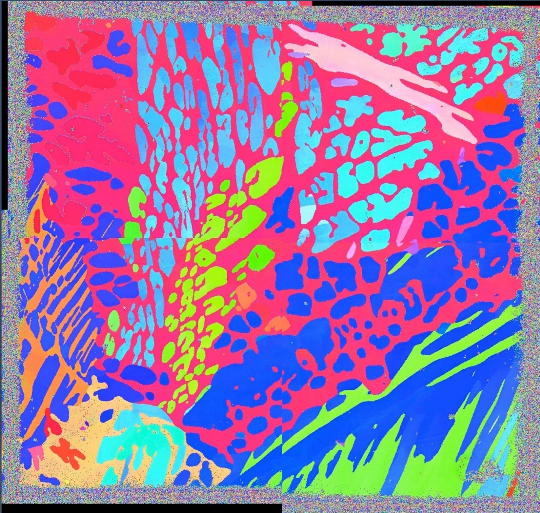
1K x 1K image with 1 micron step. 2 X 2 montage.
