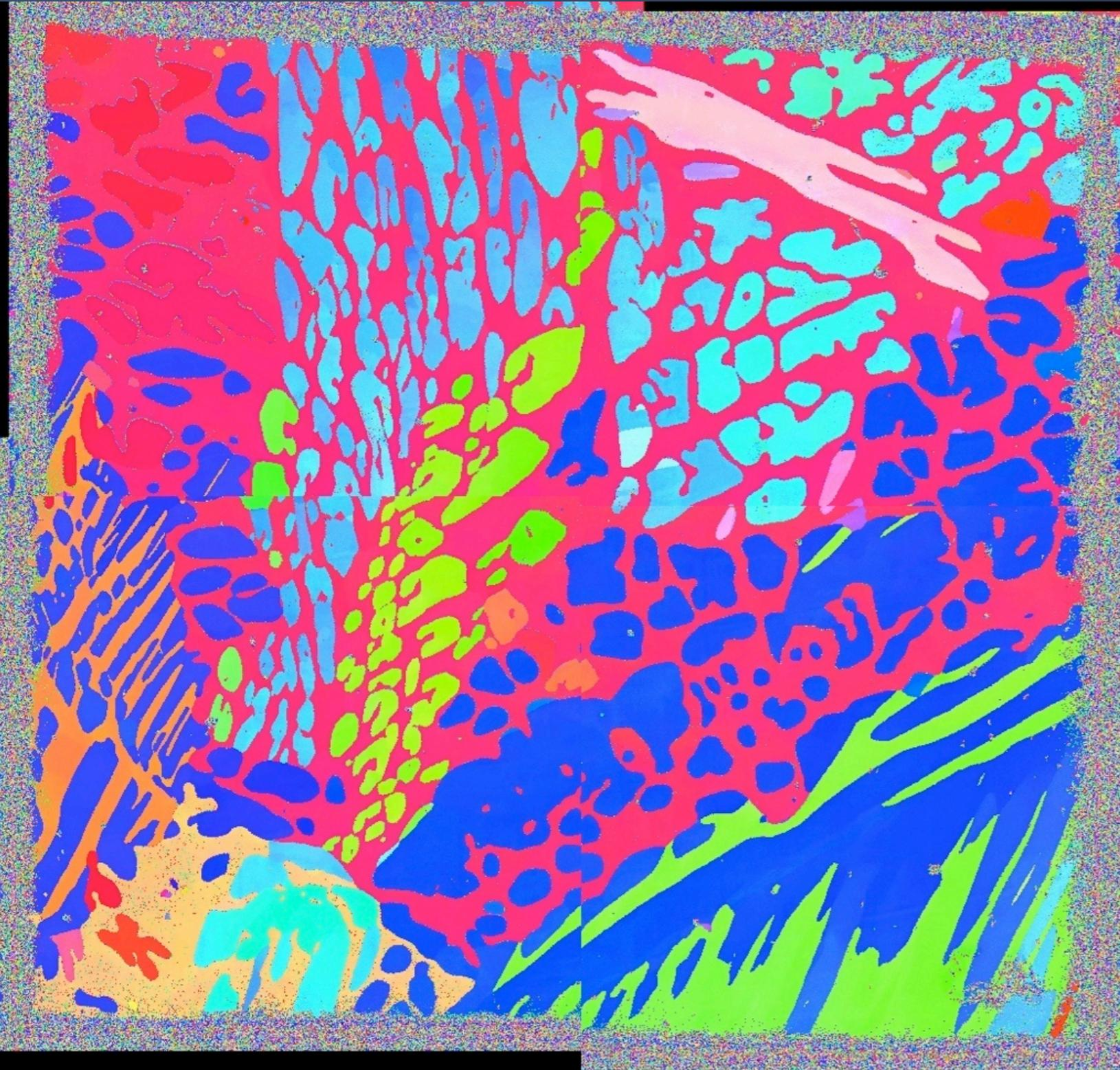
2 x 2 Combo Scan of a 2205 Duplex Stainless Steel. A 1mm laser cut grid outlines the area of interest.
