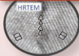
Grain boundary structure
