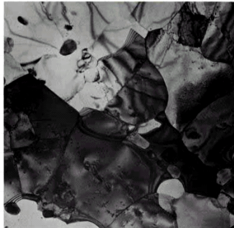
Bright-field TEM image of polycrystalline aluminum (Direct mag.: x15,000)
