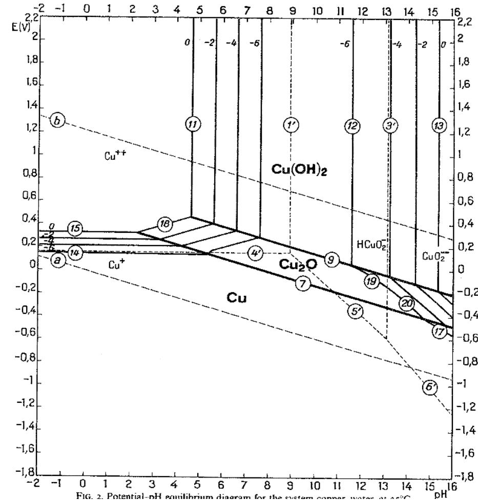
FIG. 2. Potential-pH equilibrium diagram for the system copper-water at 25°C
