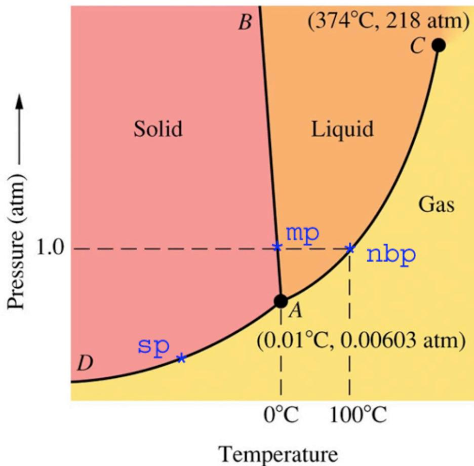
The density, viscosity, and dielectric constant of liquid water decrease as the critical point is approached.
