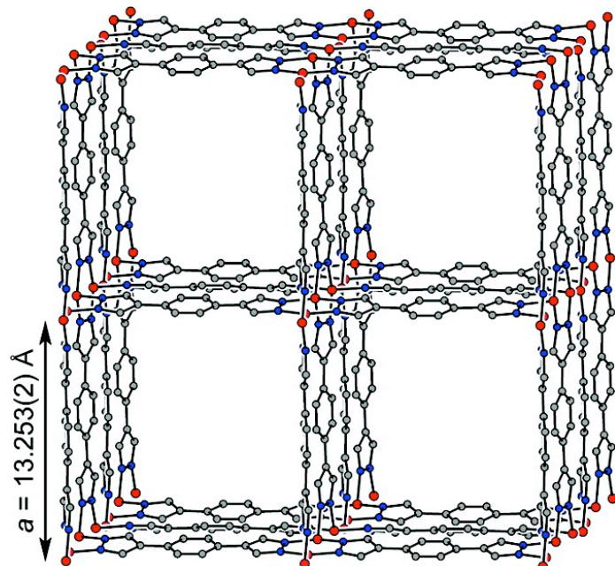
Synthesized from  $\text{Co}(\text{CF}_3\text{SO}_3)_2$  and 1,4-benzenedi(4'pyrazoyl) in diethylformamide (DEF) at 130 °C. DEF decomposes to form amines that deprotonate the ligand.
