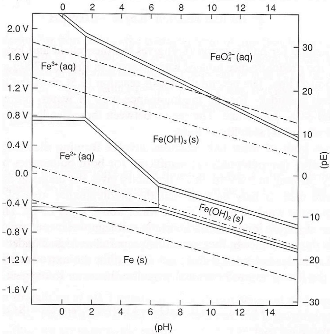
A visual representation of speciation of a metal as a function of pH and potential
