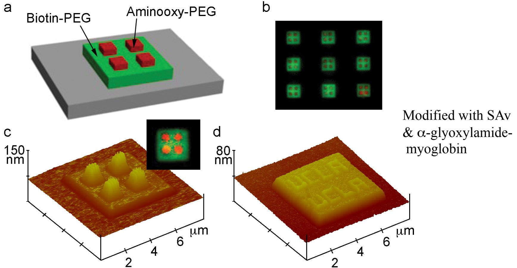
Range of multicomponent, multilayer nanoscale patterns are possible
