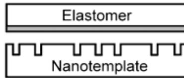
b) contact and release generates pattern by subtraction
