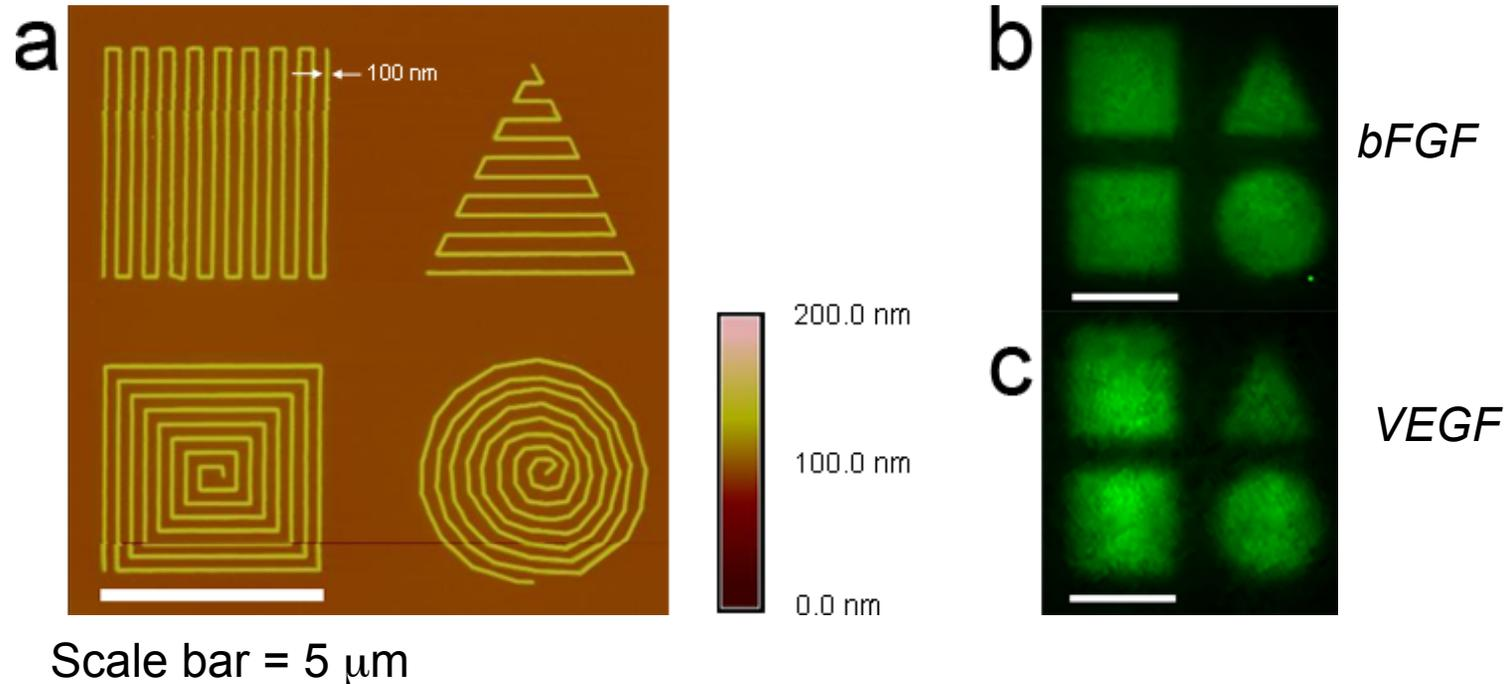
VEGF and bFGF can be patterned at the micron and nanometer scale using e-beam lithography on a heparin mimicking polymer
