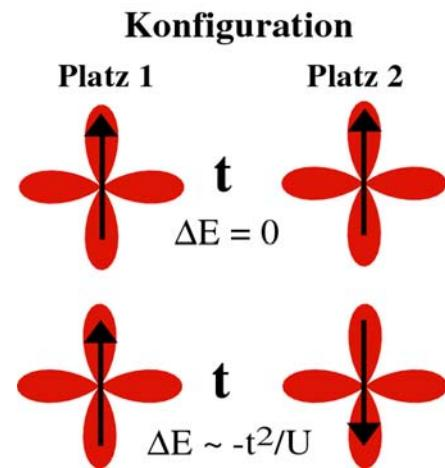
**2d-antiferromagnet,  $J/k_B \sim 1500 \text{ K}$**
