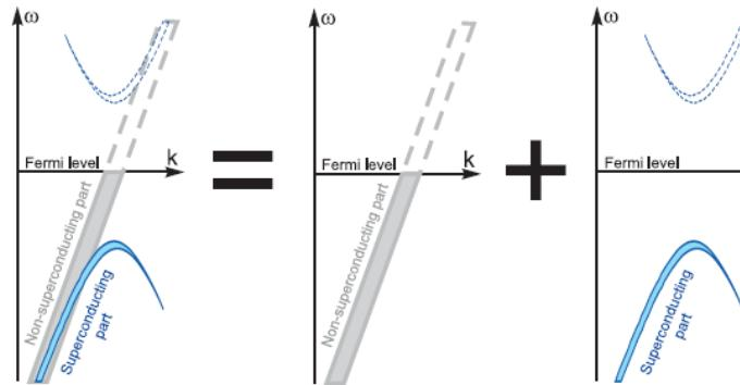
Sketch, illustrating presence of superconducting and non-superconducting components in the same spectrum. This observation supports phase separated coexistence of superconductivity and magnetism.
