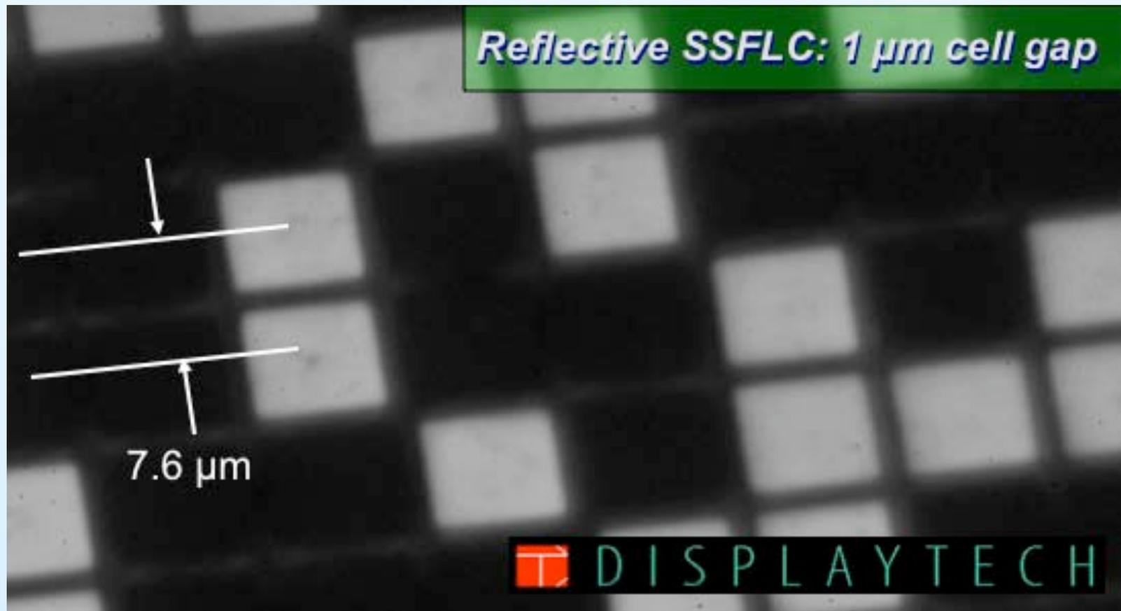
*Pixel volume as small as  $25 \mu\text{m}^3 = 25 \text{ fL} \sim 25 \text{ pg}$*
