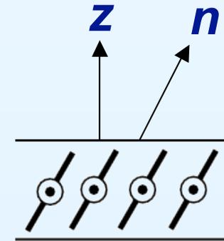
The arrows are all pointing in the same direction, and the director is tilted, giving a  $C_2$  layer structure. This symmetry is both polar and chiral.
