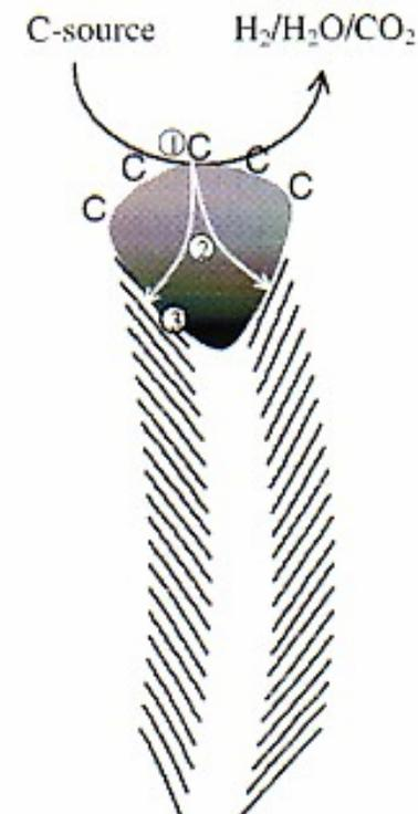
Fig. 8. Schematic representation of the catalytic growth of a CNF using a gaseous carbon-containing gas. Step 1: decomposition of carbon-containing gases on the metal surface. Step 2: carbon atoms dissolve in and diffuse through the bulk of the metal. Step 3: precipitation of carbon in the form of a CNF consisting of graphite.
