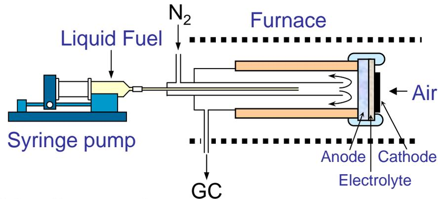
**SOFC operation on Heavy Naphtha at 700°C.**
