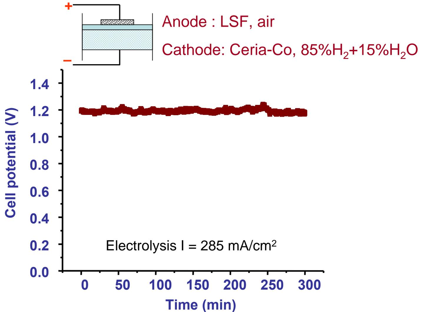
**LSF electrodes do not exhibit activation polarization and are stable during electrolysis**
