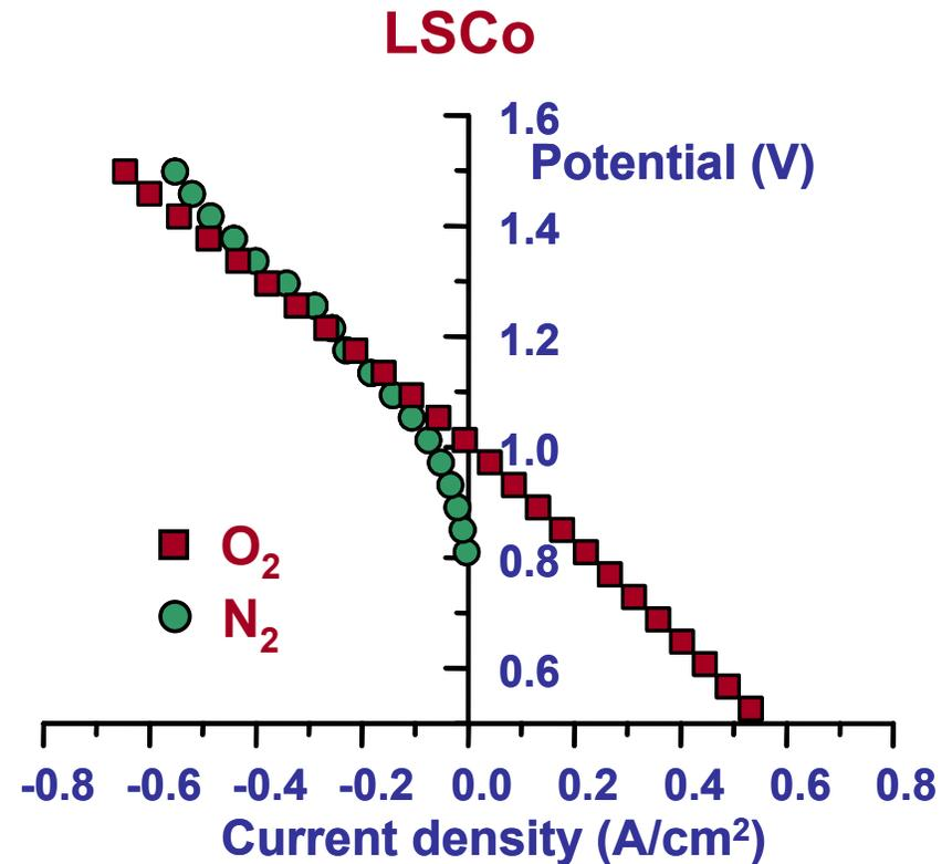
Performance of LSCo anode *increases* at high  $P_{O_2}$
