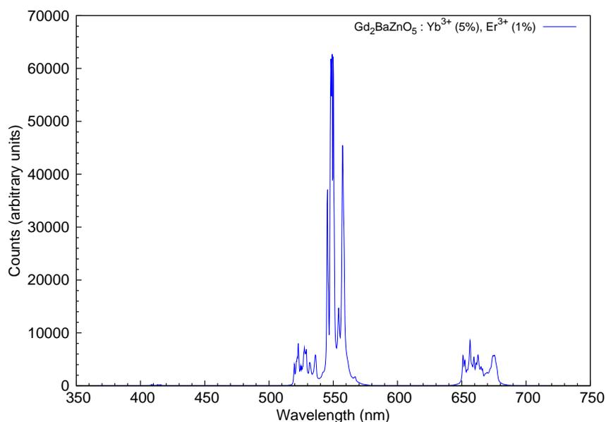
Figure 1: Up-converting spectrum of  $Gd_2BaZnO_5$  under 975nm excitation
