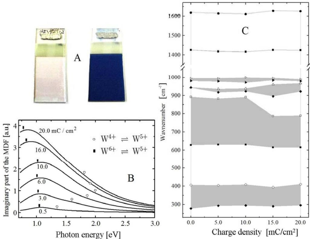
(A) Uncolored and colored tungsten oxide thin films. (B) Polaron contribution to  $Im\{\epsilon\}$  versus charge density, symbols correspond to the resonance energy position of the polaron transition. (C) IR reflection bands versus charge intercalation indicative for intercalation-induced bond reformation and polaron shift.
