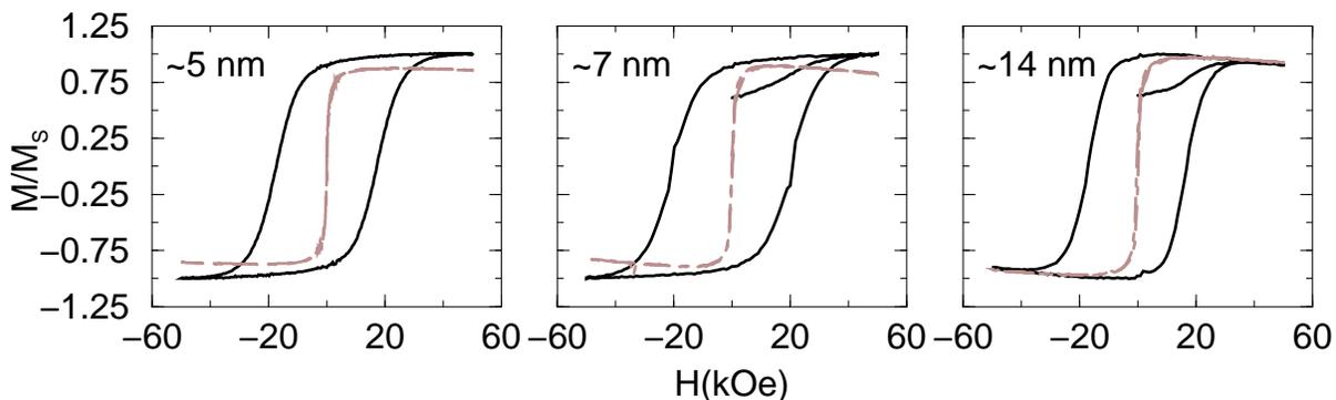
Figure 1: Hysteresis loops of three different sizes of  $\text{CoFe}_2\text{O}_4$  nanoparticles diluted in paraffin wax: the data was collected at 5 K (solid black line) and at 300 K (dashed grey line).
