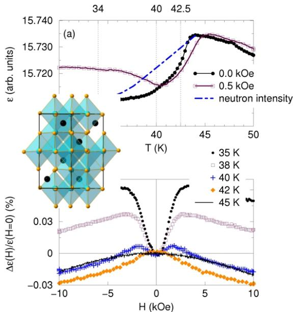
Temperature dependence of the dielectric constant, and isothermal magnetocapacitance of hausmanite  $Mn_3O_4$  which has a structure derived from a Jahn-Teller distortion of the spinel structure. The structure is depicted in the inset.
