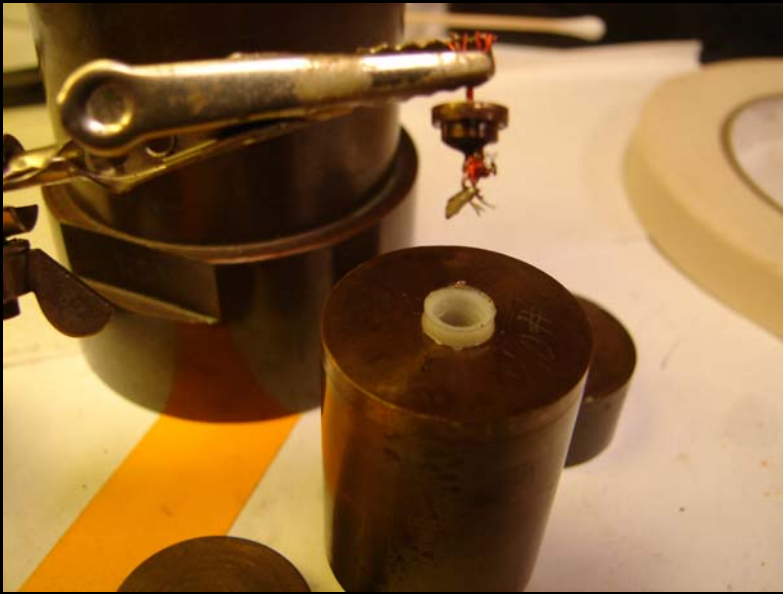
Be-Cu cap with wires, sample, and pressure gauge
