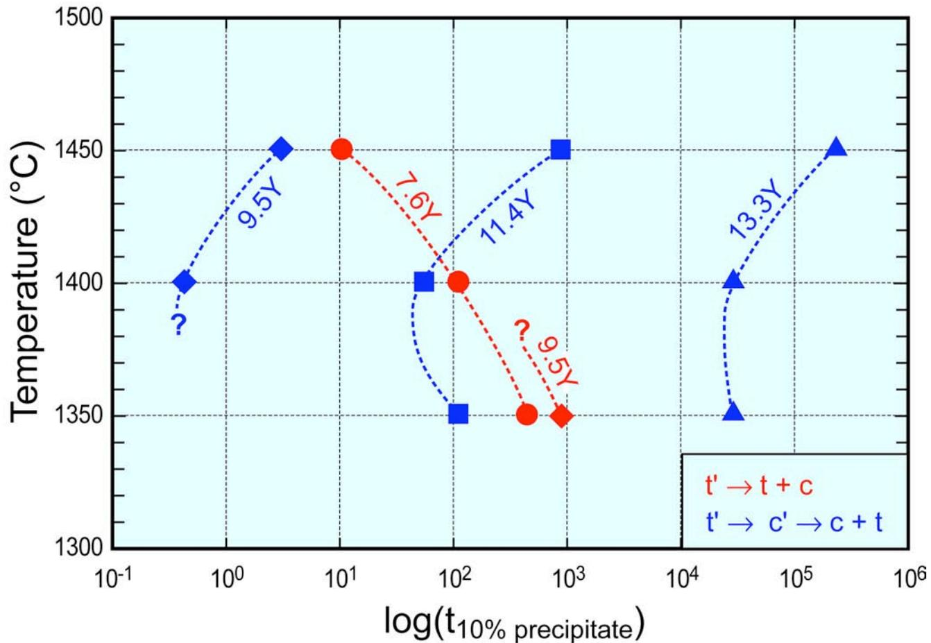
*Precipitation follows approximately AJMK kinetics but significant differences observed depending on the decomposition path*
