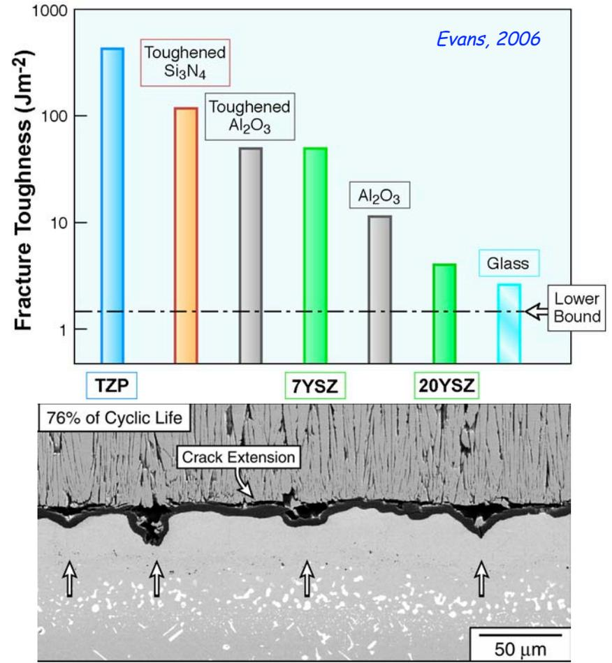
*Durability limited by crack propagation through TBC: expected to depend on toughness, which depends on Y content, but why a peak?*
