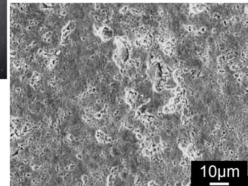
*No detectable structural changes on surface after 500 h exposure, only small depletion of Y.*
