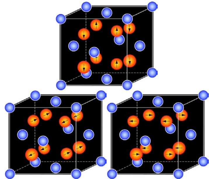
*Postulate: Variants result from ordering of anion displacements in the characteristic tetragonal pattern along each of the 3 cubic directions  $\Rightarrow t''$*
