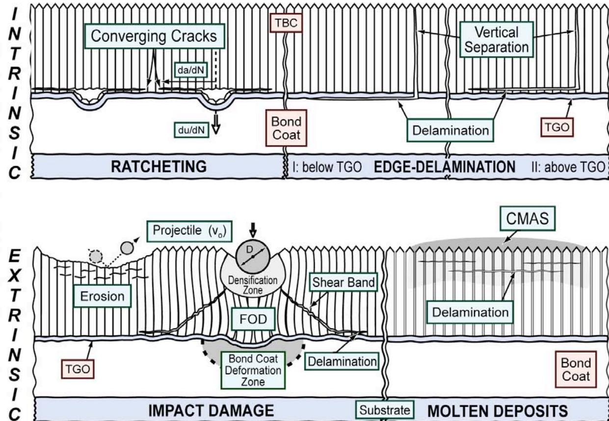
*TBCs are "live" systems, whose structure evolves over time. Predictive models must incorporate effects of evolution dynamics on damage/failure mechanisms*
