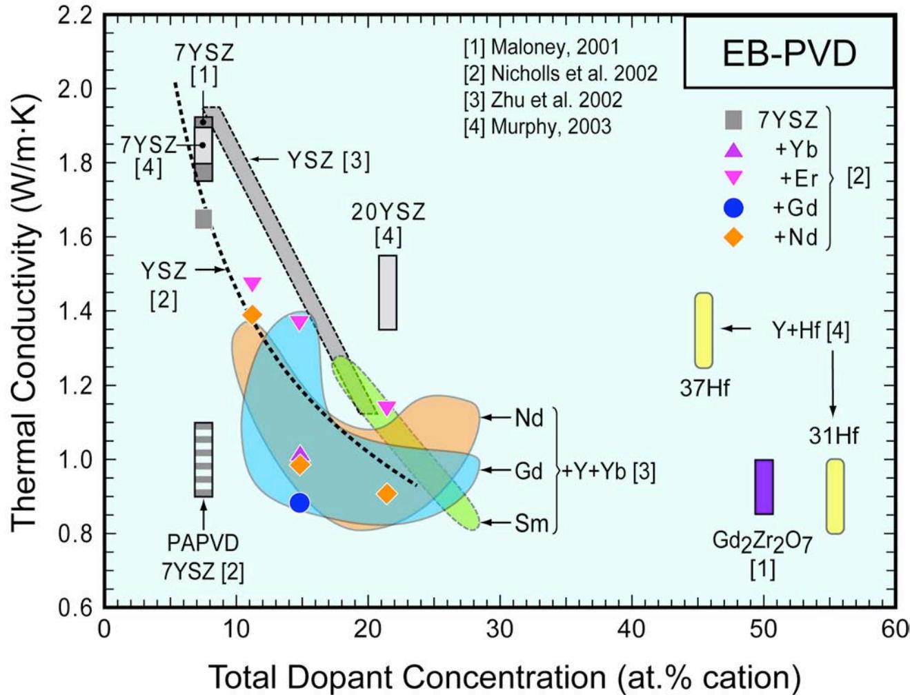
• A large variety of alternate compositions, mostly based on rare earth additions to ZrO<sub>2</sub> or YSZ, offer improved thermal insulation efficiency over 7YSZ. But...
