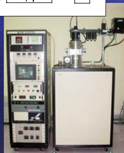
MW CVD, AX 5200 1,5 kW (Installed 2003) - Diamond thin film; Nano Diamond, DLC; Aligned CNTs
