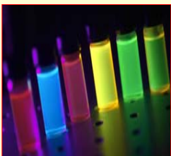
Fig 3. Composition-tunable optical properties of alloyed ZnxCd1-xSe nanocrystals with high luminescence and stability across the visible spectrum.
