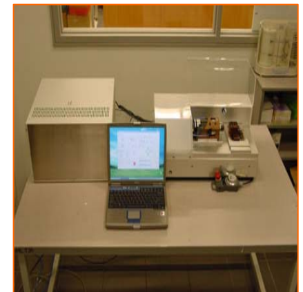
A high speed ultra precision lathe for diamond turning designed and developed in NUS
