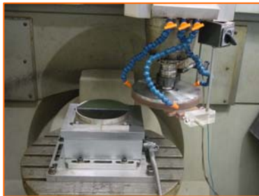
ELID Grinding setup for nano surface generation
