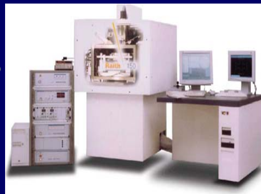
EBL --- Raith 150 Resolution: better than 50 nm
