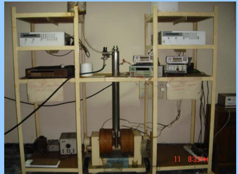
Liquid Nitrogen Cryostat (Locally Fabricated)
