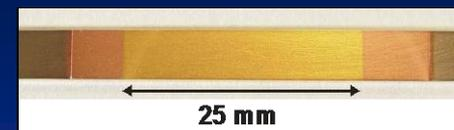
Sample showing PVD layers of 3.8  $\mu\text{m}$  Au over 35  $\mu\text{m}$  Cu layer on SS
